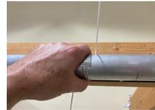
Rotate clip to tighten cord
