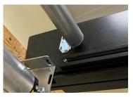
Idler tube in place above track and motor.
