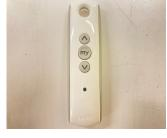
• Run motor up to raise shades: Press and hold Up arrow on remote.
