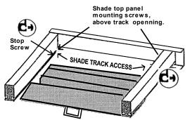
• Attach top shade panel: Load wheels of top shade panel into track through access openings and hold top hem of shade firmly against head wall or ridge above the opening. Mark mounting hole location immediately in front of and against each wheel in track. Pre-drill holes with 1/8" drill bit. Insert mounting screws so wheels are secured. There should be little to no play of top shade wheels. If there is, try using a slightly larger screw against the wheels.
