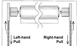
Insert the end plug into end of the shade tube opposite the clutch, pushing firmly until the plug rim meets the shade tube. IMPORTANT: If you need to remove the clutch or end plug, gently twist a screwdriver in one or more of the slots between the plastic and shade tube. Do not force the parts out as they may break. Only pry them gently.
